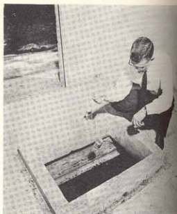
TAKING SAMPLE. Carl Webster here lowers a bottle into "Boiling Spring" to take a sample of water for careful examination. Ordinarily a heavy cast iron lid covers spring and door of spring house is kept locked
