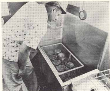
STERILIZING AT 180 DEGREES F. To meet standards of U. S. and Maryland Public Health Service all bottles are sterilized at this high temperature before being refilled. Note modern apparatus and thermometer for checking temperature
